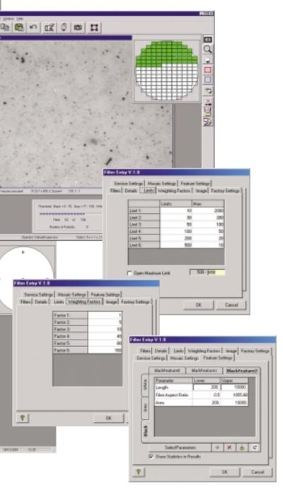
Leica QClean is designed to automatically measure circular filters with arbitrary diameters, without having to specify a scanning pattern, using a motorised microscope stage.
